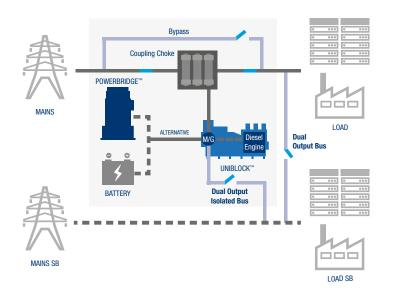
UNIBLOCK<sup>™</sup> UBTD+ with alternative Dual Output Bus configurations.
